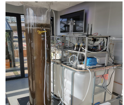
System that creates fertelizer from urine
